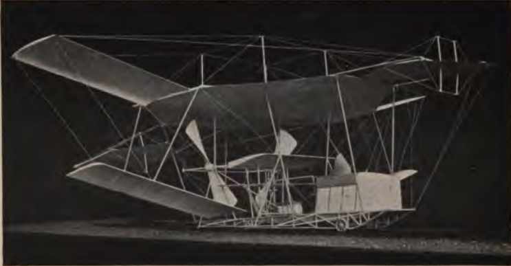
Fig. 74.—Photograph of a model of my machine, showing the fore and aft horizontal rudders and the superposed aeroplanes.
